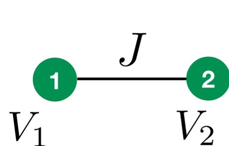
$$\hat{H} = J\hat{c}_2^\dagger\hat{c}_1 + J\hat{c}_1^\dagger\hat{c}_2 + V_1\hat{c}_1^\dagger\hat{c}_1 + V_2\hat{c}_2^\dagger\hat{c}_2$$
