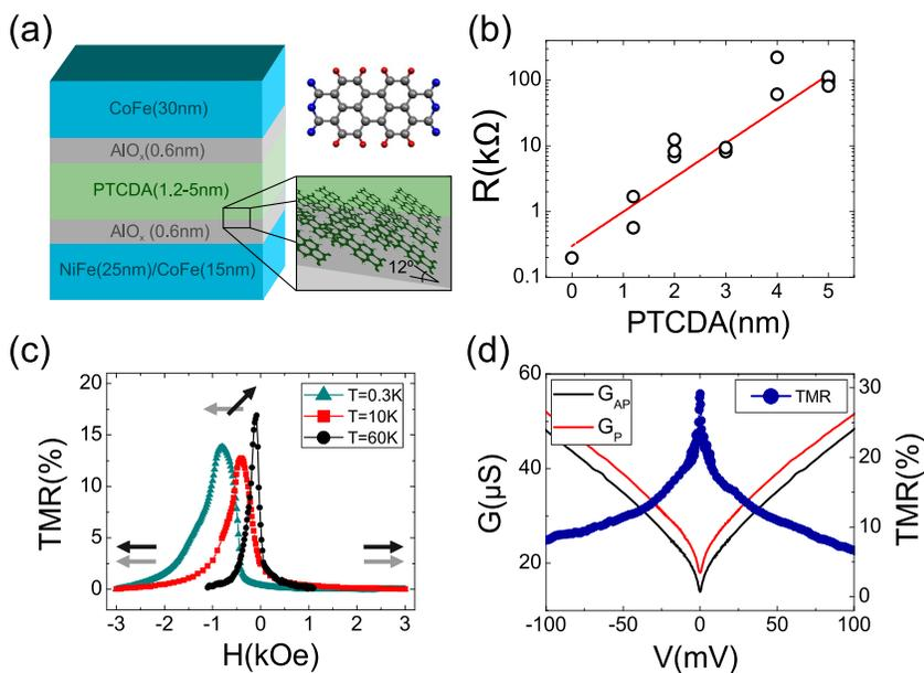
FIG. 1. (a) Sketch of the sample's layered structure. Diagram of the PTCDA molecule.<sup>37</sup> The molecules lay almost in plane, with a  $12^\circ$  tilt angle.<sup>35</sup> (b) Experimental dependence of the resistance on the PTCDA thickness. (c) TMR curves at different temperatures for a sample with 2 nm of PTCDA. (d) Dependence of the TMR and differential conductance on the bias voltage in the P and AP states for a 4 nm PTCDA O-MTJ.
