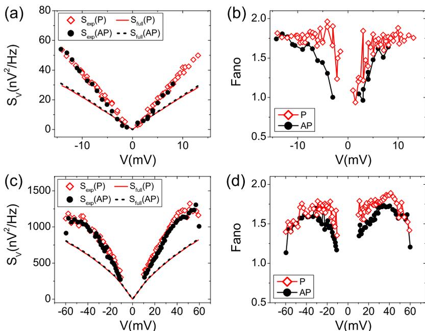
FIG. 2. Voltage dependence of the noise at  $T=0.3$  K in the P and AP states of the (a) experimental (dots) and expected full shot noise (lines) and (b) Fano factor for a 2 nm PTCDA O-MTJ. (c) and (d) present similar results for a 5 nm PTCDA O-MTJ.
