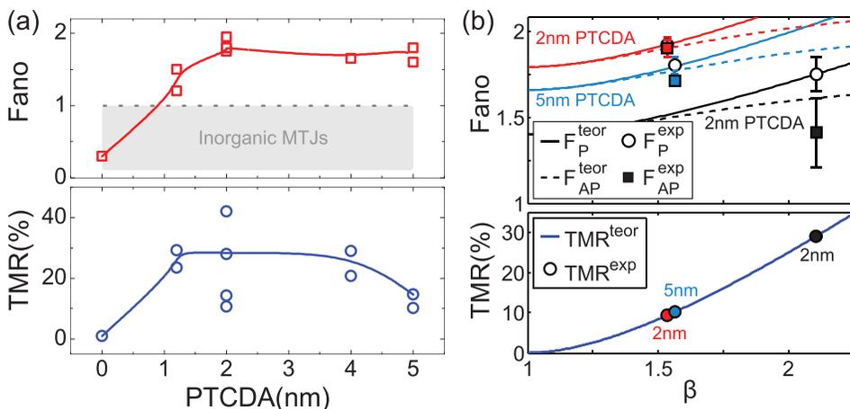
FIG. 3. (a) Maximum Fano factor in the P state and the zero bias TMR vs the PTCDA thickness, shown to be well above the range for inorganic barriers. (b) Fit of the theory to experimental values of  $F$  and TMR for the samples with 2 and 5 nm of PTCDA. The points are obtained from the average saturation value in the Fano factor vs bias plots, and the error bars indicate the dispersion of the average.
