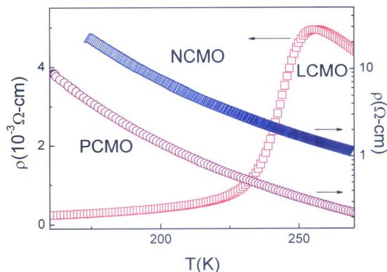
FIG. 2. (Color online) Resistivity vs temperature ( $\rho$ - $T$ ) with the left scale for LCMO and the right scale for NCMO and PCMO as indicated by arrows.
