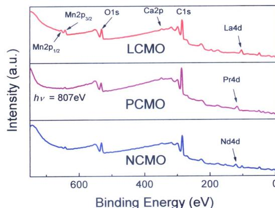
FIG. 3. (Color online) Photoemission spectra with a wide energy range for ReCMO samples, with the incident photon energy of 807 eV.
