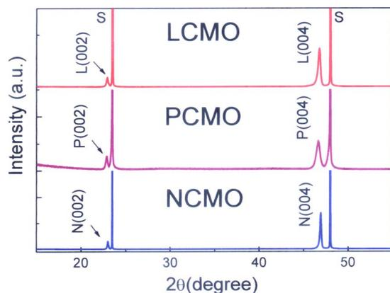
FIG. 1. (Color online) The XRD patterns of ReCMO (Re=La,Pr,Nd) thin films on LAO substrate. All lines are identified as (00 $l$ ).
