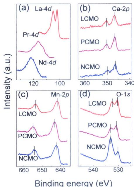
FIG. 4. (Color online) Photoemission spectra of (a) Re 4d, (b) Ca 2p, (c) Mn 2p, and (d) O 1s for various ReCMO samples.
