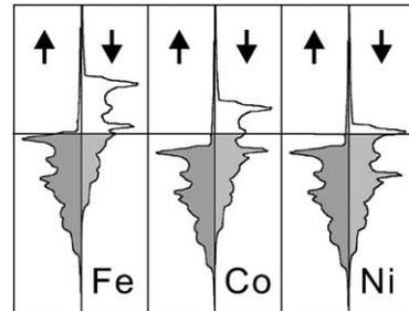
Fig. 2. Density of states for majority and minority bands in Fe, Co, and Ni. The densities of states for iron and cobalt were evaluated by taking the band shape of fcc nickel [24] modified with the spin splitting proportional to magnetic moment in accordance with the Stoner theory [23].
