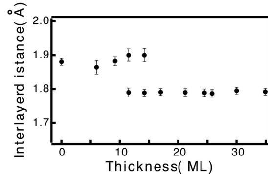
FIG. 3. The interlayer distances  $d_{\perp}$  deduced from the LEED- $I/V$  curves of  $n$  ML Mn/ $\text{Cu}_3\text{Au}(100)$ .
