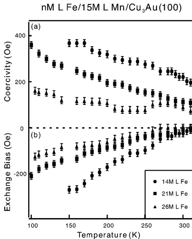
FIG. 5. Variation of (a)  $H_c$  and (b)  $H_e$  for 14, 21, and 26 ML Fe/15 ML Mn/Cu<sub>3</sub>Au(100) with increasing temperature.
