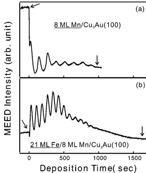
FIG. 1. (a) and (b) are the MEED oscillation curves of 8 ML Mn grown on  $\text{Cu}_3\text{Au}(100)$  and subsequently 21 ML Fe grown on 8 ML Mn/ $\text{Cu}_3\text{Au}(100)$ . The arrows indicate the time for shutter opening and closing.
