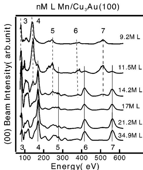
FIG. 2. LEED- $I/V$  curves of  $n$  ML Mn/ $\text{Cu}_3\text{Au}(100)$ . Solid lines and dashed lines indicate two series of peaks. The numbers are the indices denoting the integer numbers of the single scattering Bragg interference condition (Refs. 9,10).
