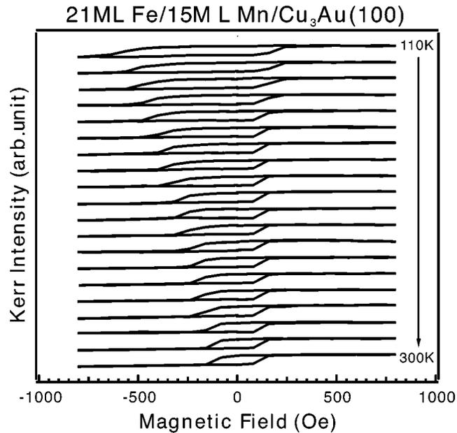
FIG. 4. Longitudinal MOKE hysteresis loops of 21 ML Fe/15 ML Mn/Cu<sub>3</sub>Au(100) with increasing temperature from 110 to 300 K ( $\Delta T = 10$  K).
