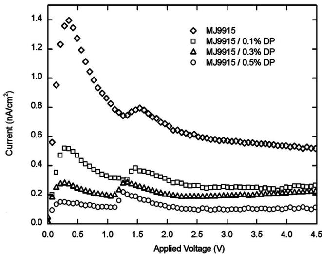
FIG. 2. Transient currents through the TN MJ9915 and MJ9915/DP cells under the applied dc voltage.
