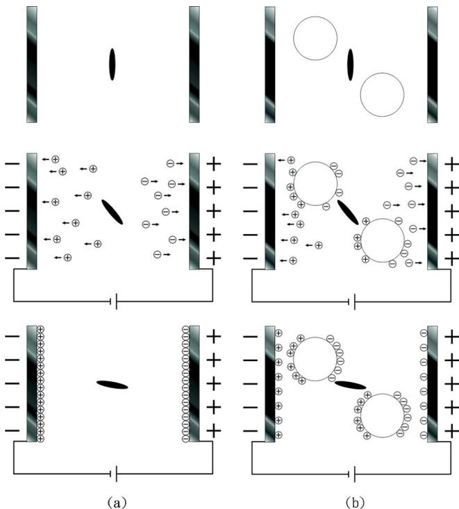
FIG. 3. Conceptual depiction variation of internal ions in a TN cell. (a) Without doping of diamond powders and (b) with doping of diamond powders.
