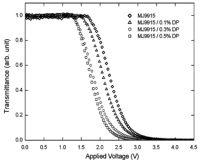
FIG. 4. Power transmitted through the TN MJ9915 and MJ9915/DP cells under the applied dc voltage.
