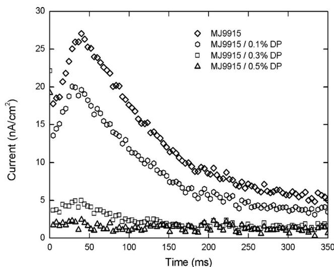
FIG. 1. Transient currents induced by a dc voltage of 1.2 V applied to an MJ9915 cell and three MJ9915/DP cells at room temperature.
