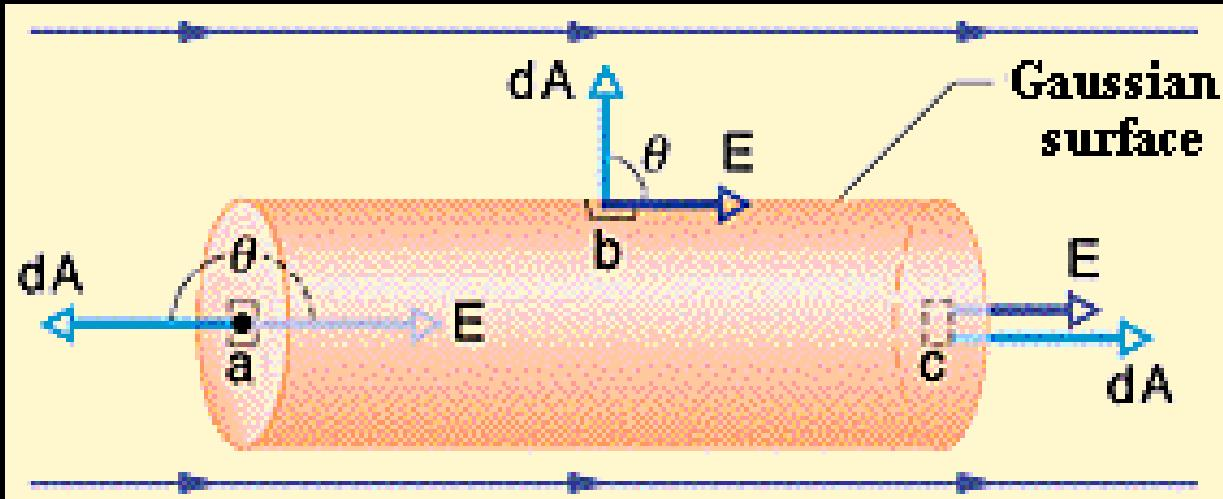
$$\begin{aligned}\Phi &= \oint \vec{E} \cdot d\vec{A} \\ &= \int_a \vec{E} \cdot d\vec{A} + \int_b \vec{E} \cdot d\vec{A} + \int_c \vec{E} \cdot d\vec{A} \\ &= -EA + 0 + EA = 0\end{aligned}$$
