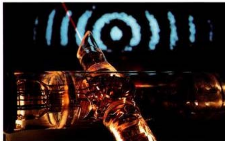
NIST-7 atomic fountain Currently, the most accurate timekeeping device is a type of atomic clock called the "atomic fountain," which tunes into the spin transition frequency of cesium-133 atoms, as do other atomic clocks. Its greater accuracy is obtained by using lasers to trap and cool a "pocket" of cesium atoms to just above absolute zero (the lowest possible temperature). The latest model, the NIST-F-1, is accurate to one second in 20 million years.
