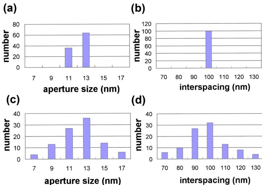
FIG. 4. The statistical analysis for two growth modes: (a) Aperture size distribution in FIB-guided area; (b) interspacing distribution in FIB-guided area; (c) aperture size distribution in self-organized area; and (d) interspacing distribution in self-organized area.
