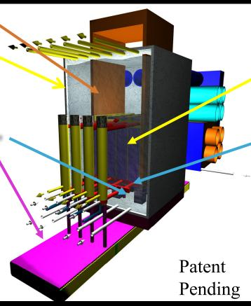
If over-heated, fuel salt expands out of reaction zone. Online distillation of fission products. Circulate until 100% burn-up. Spill: Nal, CsF, SrF<sub>2</sub> in salt that freezes in 10 s.
