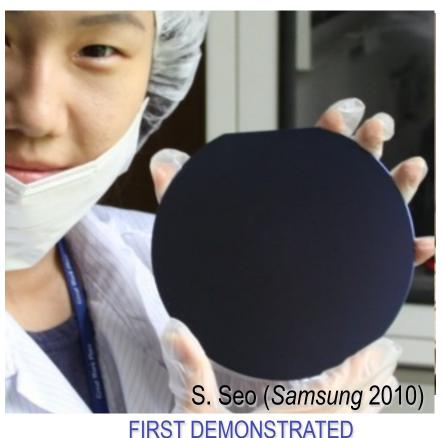
graphene-on-Si wafers uniform; no multilayer regions; few cracks; µ >5,000 cm²/Vs
