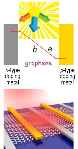
ballistic transport of photo-generated carriers in built-in electric field
