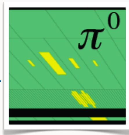
⇐ The Atlas calorimeter has fine  $\eta$  segmentations (4mm strips) can well separate  $\pi^0$  and photon.
