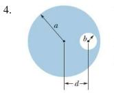
The figure to the left shows a cross section of a long cylindrical conductor of radius a = 4.00 cm containing a long cylindrical hole of radius b = 1.50 cm. The central axes of the cylinder and hole are parallel and are distance d = 2.00 cm apart; current i = 5.25 A is uniformly distributed over the tinted area. (a) What is the magnitude of the magnetic field at the center of the hole? (10%) (b) Show that the magnetic field in the hole is uniform. (10%)
